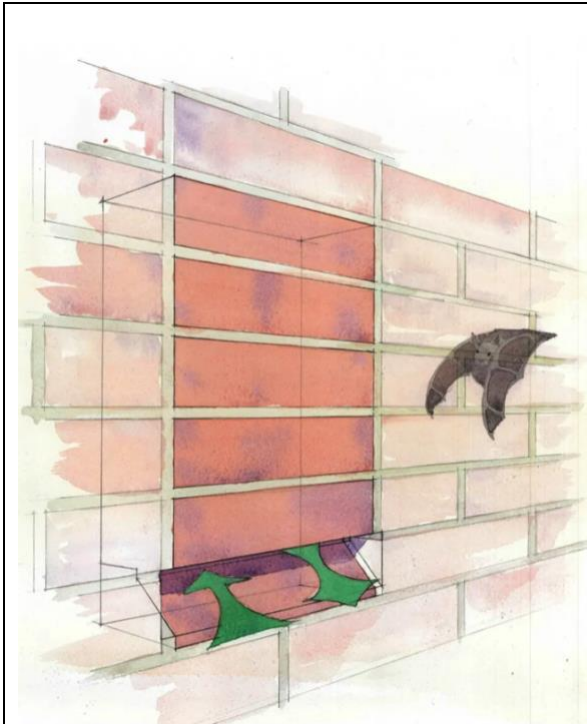
Figure 22.9 – Bat brick showing access
