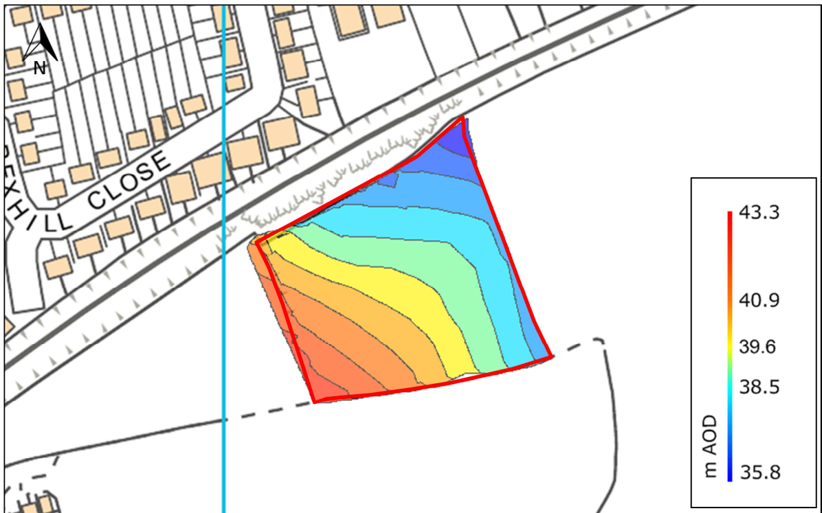
Figure 2: Digital Terrain Model from Topographical Survey
