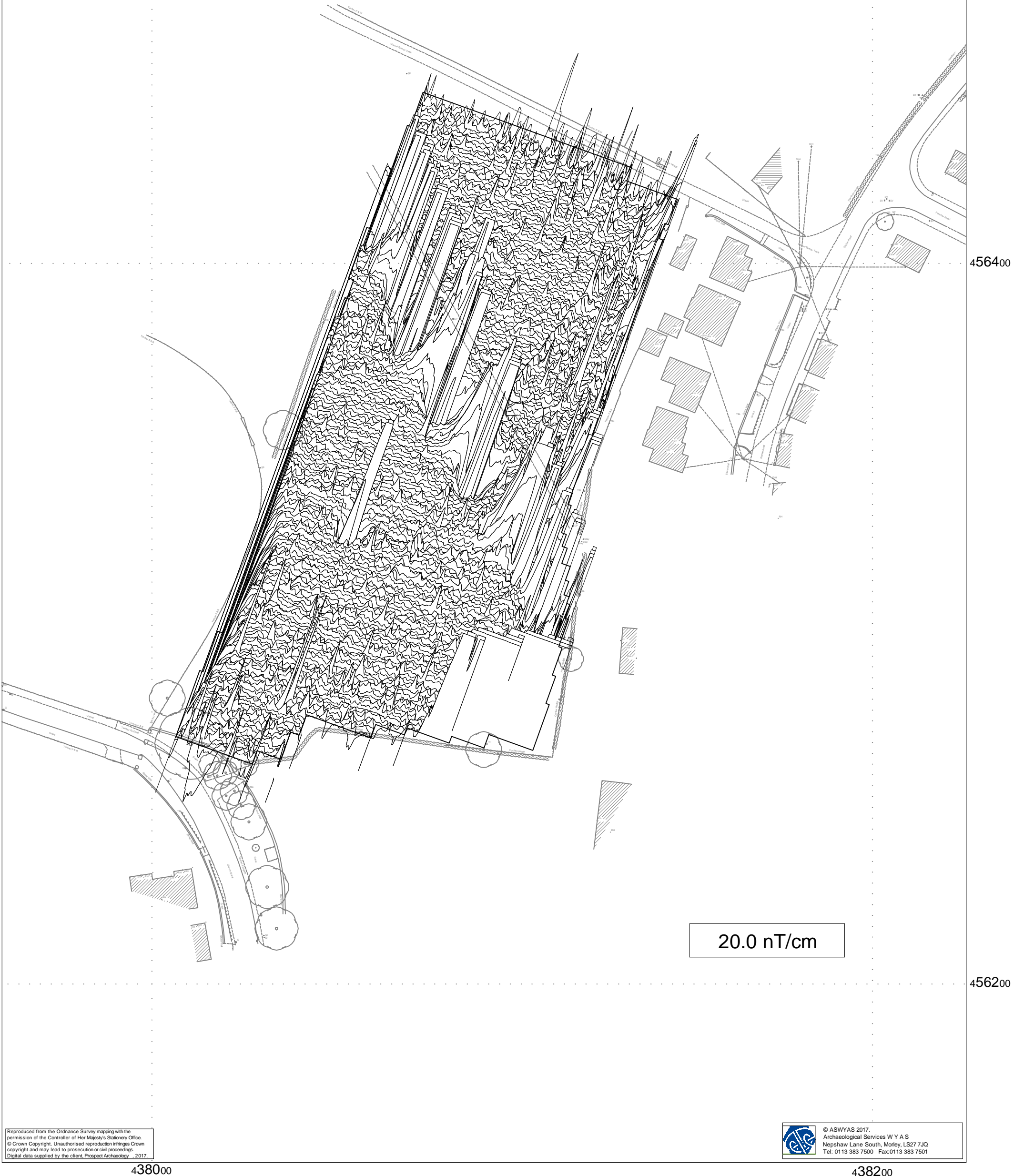
Fig. 4. XY trace plot of minimally processed magnetometer data (1:1000 @ A3)
